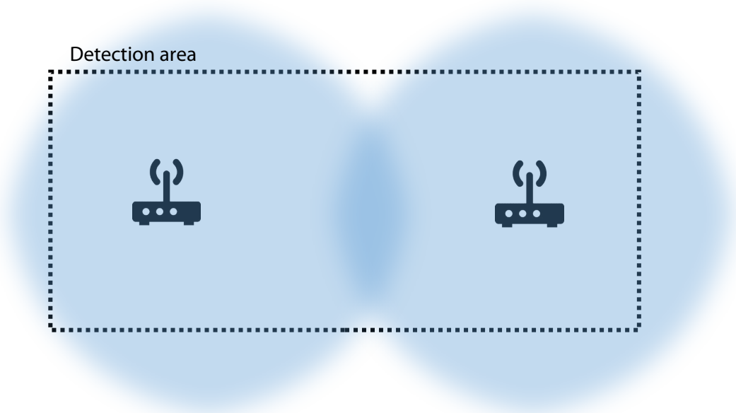
Figure 12 - use multiple receivers to cover the detection area in case the detection area is not square, or circle shape.
