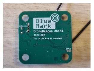
Figure 1 - DroneBeacon db151 (left) and db151pcb (right) transponders. Picture on the bottom shows the external connectors of the db151pcb (power and status aux and GPS out)
