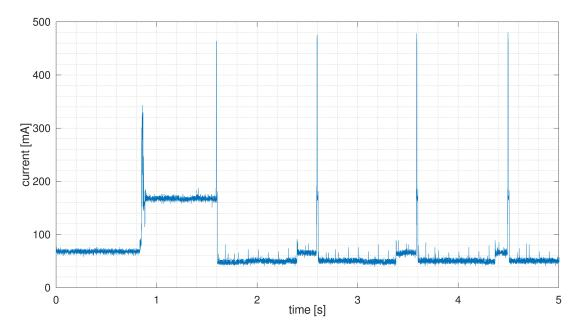
Figure 7 - Current profile of the db151/db151pcb transponder in default configuration (WLAN Beacon) (input voltage +5V)
