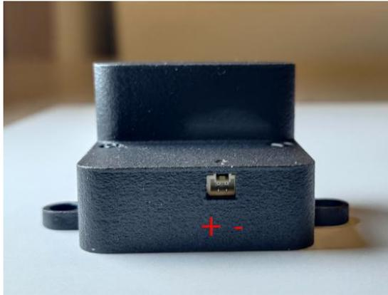
Figure 2 - Power connector the + signs indicates pin 1 and need to be connected to the input voltage.
